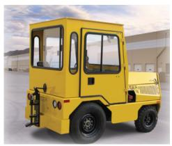
The TC-30/60 tow tractor is designed to provide a versatile and highly maneuverable solution for your towing requirements demanding 3,000-6,000 pounds (13.3-26.7 kN) of drawbar pull.
